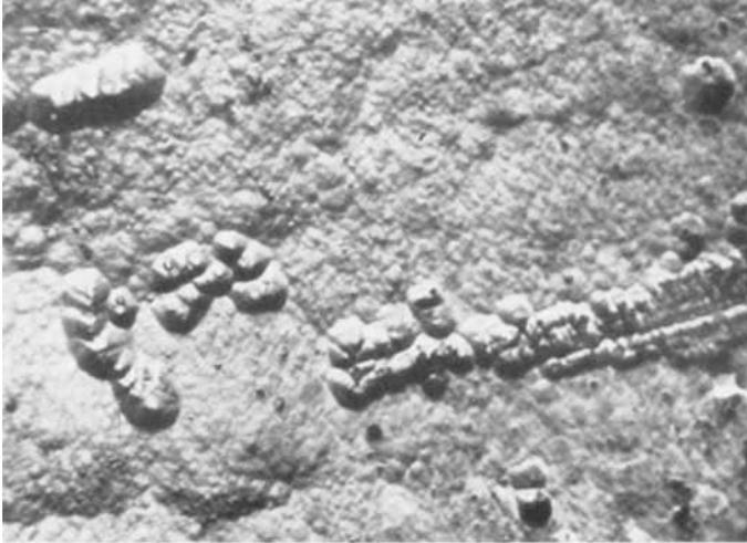
*Fig. 6 Deposits of graphite on the surfaces of single crystal ruthenium-carbon alloys:*
