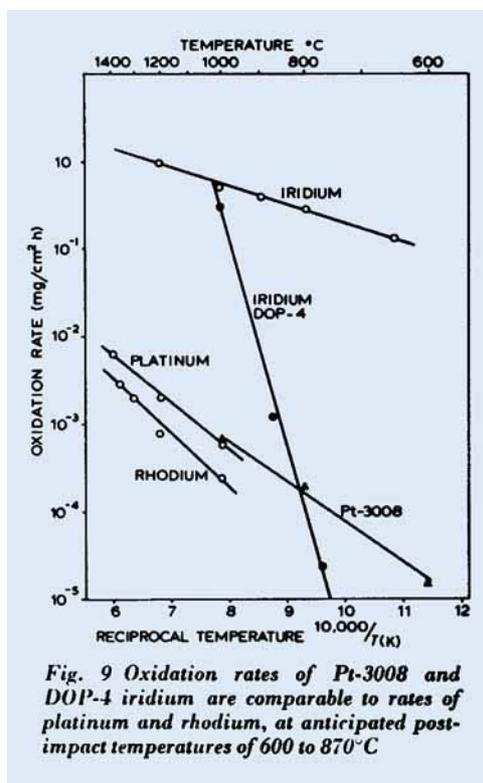
Fig. 9 Oxidation rates of Pt-3008 and DOP-4 iridium are comparable to rates of platinum and rhodium, at anticipated post-impact temperatures of 600 to 870°C
