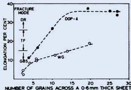
**Fig. 6** The impact ductility of DOP-4 iridium at 85 m/s is greater than that of undoped Ir-0.3%W (WG) at 1350°C because of the presence of thorium and aluminium. The ductility of both alloys is sensitive to the grain size. Sheet thickness is 0.6 mm. DR=ductile rupture, TF=transgranular fracture, GBS=grain boundary separation
