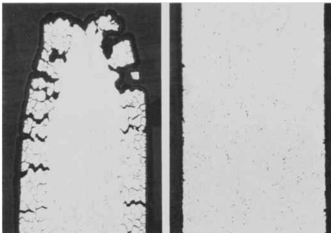
*Fig. 8 Cross-section of Pt-3008 oxidised in still air at 800°C. (Left) Surface embrittlement due to oxygen diffusion down grain boundaries after 1000 h exposure. (Right) Tungsten-rich particles after 3000 h exposure embrittle alloy, for the effect of this on some physical properties see Figure 7 × 65*
