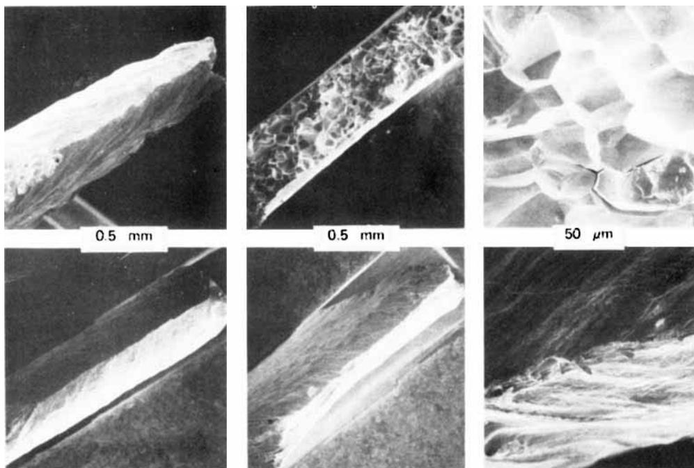
*Tensile test at 1093°C and 85 μm/s Impact test at 1250°C and 85 m/s Impact test at 1250°C and 85 m/s*
