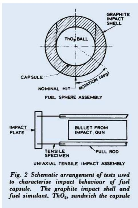
**Fig. 2 Schematic arrangement of tests used to characterise impact behaviour of fuel capsule. The graphite impact shell and fuel simulant,  $\text{ThO}_2$ , sandwich the capsule**
