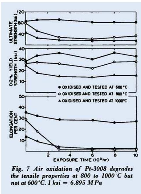
shown in Figure 8. This result, expected from the studies of Betteridge (24) and Chaston (25), represents the trade-off between increasing the strength and melting temperature of the alloy and lowering its oxidation resistance. In contrast, these characteristics are not observed in iridium alloys. The tensile properties of iridium-0.3 per cent tungsten
