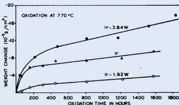
Fig. 10 Iridium and Ir-W alloys exhibit transient oxidation behaviour up to about 200 h of air exposure at 770°C
