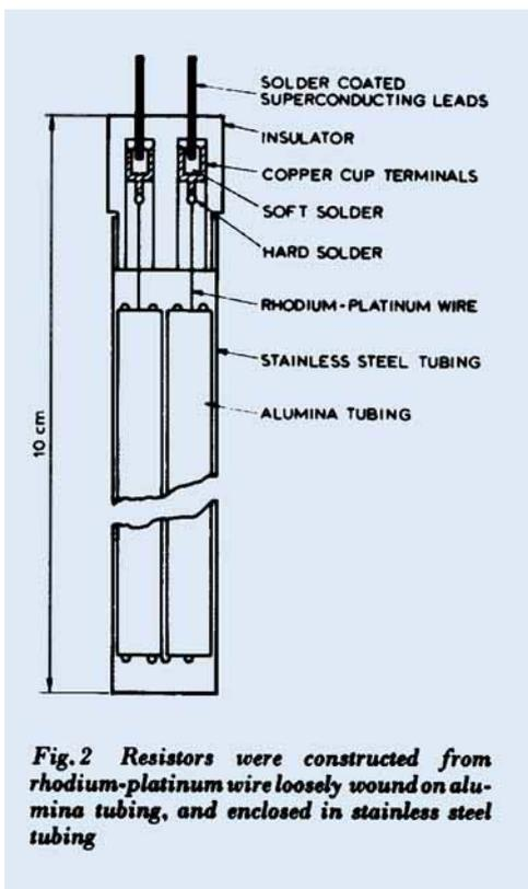
**Fig. 2** Resistors were constructed from rhodium-platinum wire loosely wound on alumina tubing, and enclosed in stainless steel tubing
