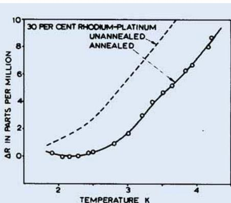
**Fig. 3** The change in resistance,  $\Delta R$ , of a 30 per cent rhodium-platinum resistor, in the annealed and unannealed condition, was determined in the temperature range 1.9 to 4.2K
