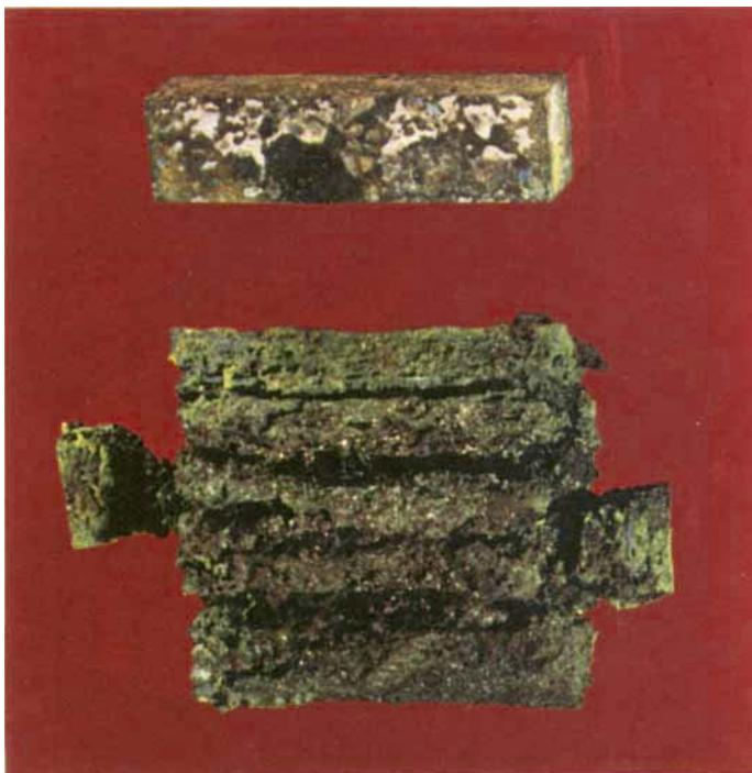
*Fig. 6 Salt shower testing at 800°C demonstrates the superior corrosion resistance of the platinum-containing RJM1020 alloy (top), compared to that of Mar-M200 (bottom), a conventional superalloy. The platinum-containing alloy was subjected to the corrosive environment for 300 hours but testing of the conventional superalloy was terminated after 100 hours. Prior to testing both specimens were the same shape and size*
