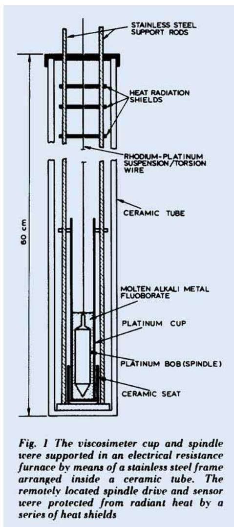
*Fig. 1 The viscosimeter cup and spindle were supported in an electrical resistance furnace by means of a stainless steel frame arranged inside a ceramic tube. The remotely located spindle drive and sensor were protected from radiant heat by a series of heat shields*
