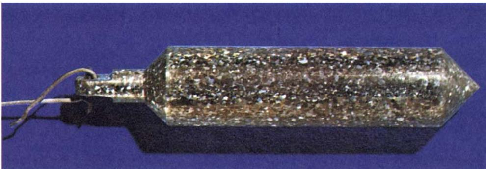
*Fig. 2 The viscosimeter spindle, which weighed approximately 60 g, was machined from a solid piece of platinum to a diameter of 1 cm and an overall length of 4.3 cm, while the internal diameter of the cup was 1.25 cm and the depth 12 cm. The finely etched surface texture seen on the platinum resulted from attack by the molten alkali metal fluoborate but it had no effect on the viscosity measurements*
