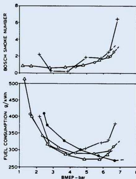
Fig. 3 The performance results obtained from a Catalytic Comet engine are compared with those obtained from other engines of similar cylinder size. The figures are extrapolated to brake performance of four cylinder engines. All engines at all loads were set for best economy. Engine speed 1500 rpm
