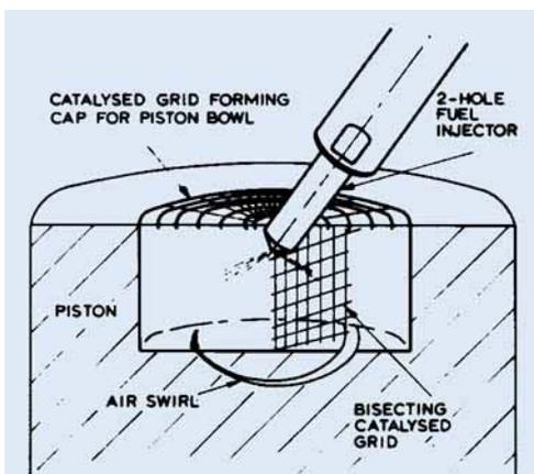
*Fig. 1 Two platinised catalyst grids are used to initiate combustion in the combustion chamber of a Direct Injection diesel engine. Air and fuel are mixed together as they swirl through half a revolution of the piston bowl before being oxidised as they pass through a vertical catalyst grid; any unoxidised fuel being consumed as it passes through a second grid*
