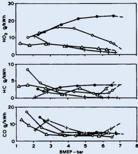
Fig. 4 The exhaust emissions from a Catalytic Comet engine are compared with those from various engines of similar cylinder size. The figures are extrapolated to brake values of four cylinder engines. All engines at all loads were set for best economy. Engine speed 1500 rpm
