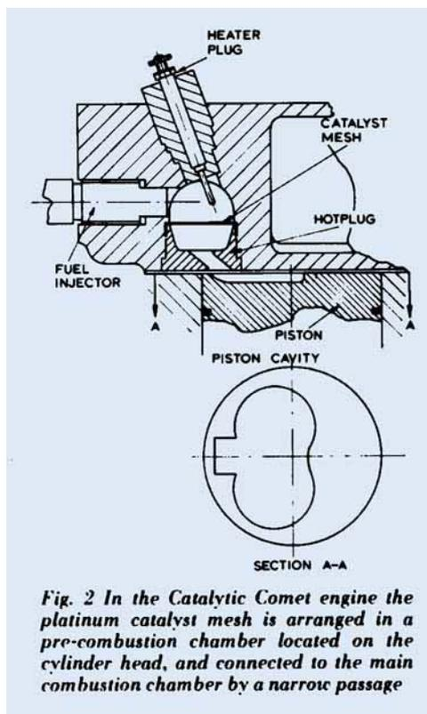
*Fig. 2 In the Catalytic Comet engine the platinum catalyst mesh is arranged in a pre-combustion chamber located on the cylinder head, and connected to the main combustion chamber by a narrow passage*
