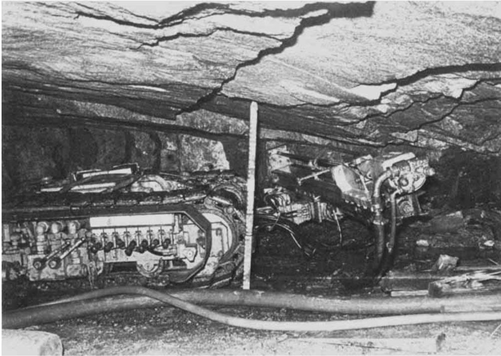
*Fig. 4 Rigs mounted on crawler tracks and powered by compressed air have been designed and built to Rustenburg Platinum Mines' own specification to facilitate mechanical drilling in very narrow stopes. The sophisticated drilling rig shown here enables a highly trained, skilful operator to increase his productivity by over 300 per cent and has demonstrated its mechanical reliability and economic viability for drilling the hard rock of the Merensky Reef*
