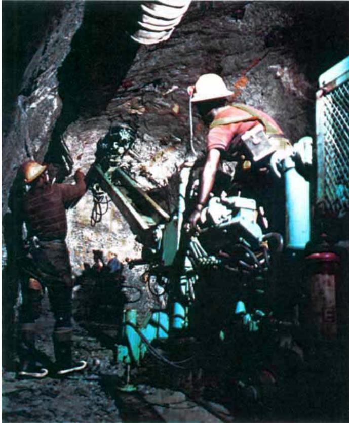
*Fig. 2 Single or multi-boom rigs are now in general use for drilling the holes which carry the blasting explosives during haulage development. The introduction of such rigs has improved working conditions and reduced operator fatigue, and has contributed to increased productivity*
