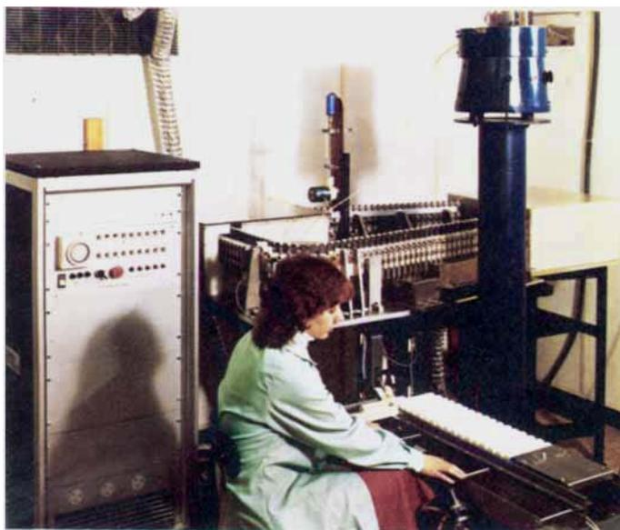
*Fig. 1 Ceramic substrates are delivered by a vibratory feed system to an endless chain conveyor that carries them through both the dipping stage, where the platinum film is deposited, and the subsequent drying operation. Next, the coated substrates are automatically loaded on to refractory kiln furniture ready for firing*
