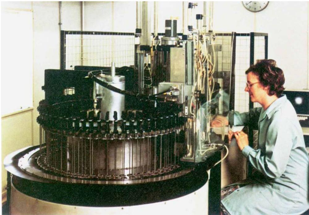
*Fig. 4 Key electrical properties are determined as the devices are compared with standards separately in ice and steam baths. The resulting data is processed by an on-line computer which grades the devices, and displays and records the key property values*
