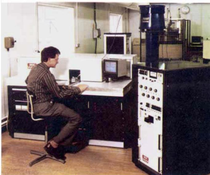
*Fig. 2 The resistance path is defined by a pattern of lines burnt through the platinum film by a high intensity laser beam. This is controlled by an on-line computer to provide the requisite accuracy. The whole operation can be observed by a close circuit television system*
