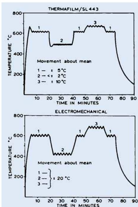
**Fig. 8** A comparison between the performance of an electronic and an electro-mechanical system illustrates the advantages of the former. The temperature indicated is that measured on the surface of a glass ceramic top cooker panel by a standard measuring system. The conditions were: 1 Free radiation, 2 Aluminium pan with a ground base 15 cm diameter containing one litre of water, and placed centrally on the hot area of the cooker, 3 Empty milk pan 11 cm diameter, concave base placed centrally
