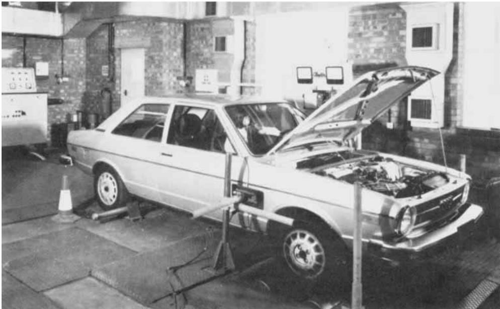
*Fig. 2 A vehicle is driven on a rolling road dynamometer over a driving cycle that simulates a typical urban driving schedule and exhaust gas is continuously sampled and collected. The gases collected are analysed for hydrocarbons, carbon monoxide and nitrogen oxides. This is known as the C.V.S. test and is used to assess the ability of a vehicle to meet legislated standards over 50,000 miles*
