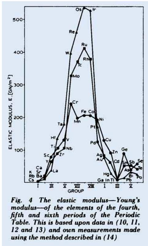
Fig. 4 The elastic modulus—Young's modulus—of the elements of the fourth, fifth and sixth periods of the Periodic Table. This is based upon data in (10, 11, 12 and 13) and own measurements made using the method described in (14)
