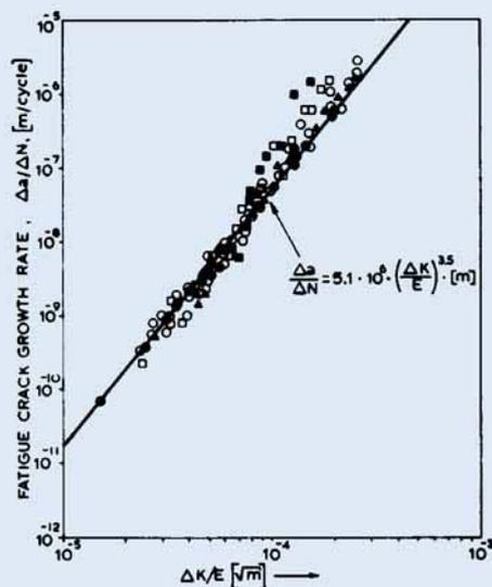
**Fig. 3** The fatigue crack growth rates of Figure 2 are plotted here against  $\Delta K/E$ . Note how well  $\Delta K/E$  normalises the fatigue crack growth rates in different metals
