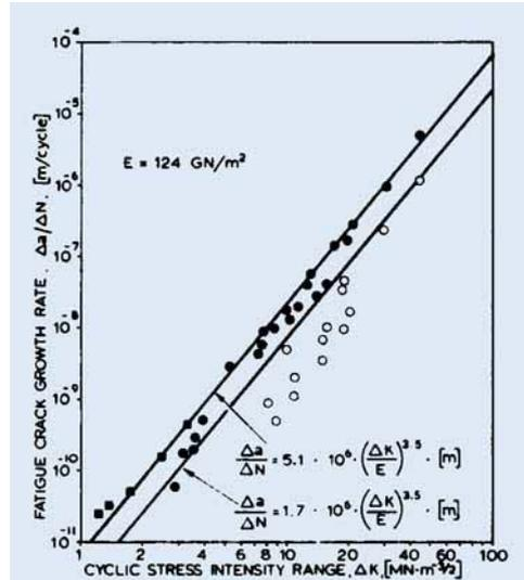
Fig. 5 The effect of stress intensity and environment on the growth rate of fatigue cracks in cold rolled pure palladium. Sinusoidal wave load at 23°C. The lines represent the predictions of Equations (iii) and (iv)
