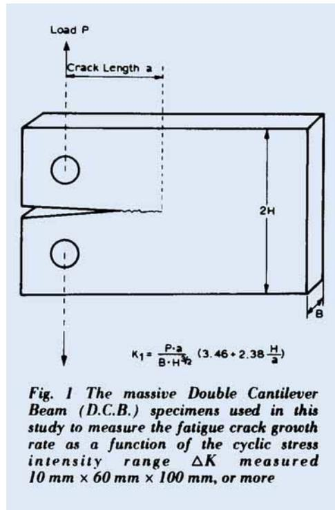
*Fig. 1 The massive Double Cantilever Beam (D.C.B.) specimens used in this study to measure the fatigue crack growth rate as a function of the cyclic stress intensity range  $\Delta K$  measured 10 mm  $\times$  60 mm  $\times$  100 mm, or more*
