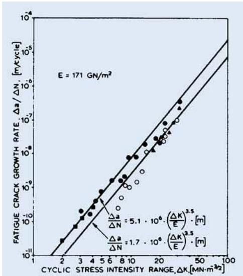
**Fig. 6** The effect of stress intensity and environment on the growth rate of fatigue cracks in cold rolled pure platinum. The lines represent the predictions of Equations (iii) and (iv)
