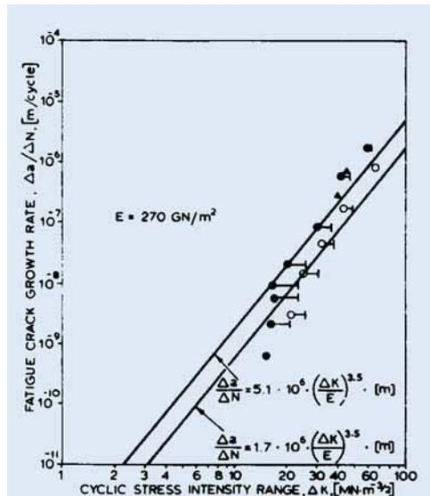
**Fig. 7** The effect of stress intensity and environment on the growth rate of fatigue cracks in a cold rolled 30 per cent rhodium-platinum alloy. The lines represent the predictions of Equations (iii) and (iv)
