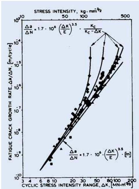
**Fig. 9** The effect of stress intensity on the fatigue crack growth rates in a 12 per cent chromium-0.2 carbon stainless steel exposed to vacuum. Certain heat treatments embrittle the steel, and in such cases the correction factor  $\frac{K_C}{K_C - \Delta K}$  describes the acceleration of fatigue cracks as the cyclic stress intensity range,  $\Delta K$ , approaches the fracture toughness  $K_C$ . Conditions:  $10^{-3}$  torr, 2.3 hertz,  $R = 0$
