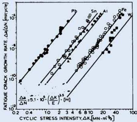
**Fig. 2** Effect of the cyclic stress intensity range,  $\Delta K$ , on the fatigue crack growth rates, in air, in a series of metals with vastly different moduli of elasticity,  $E$ .
