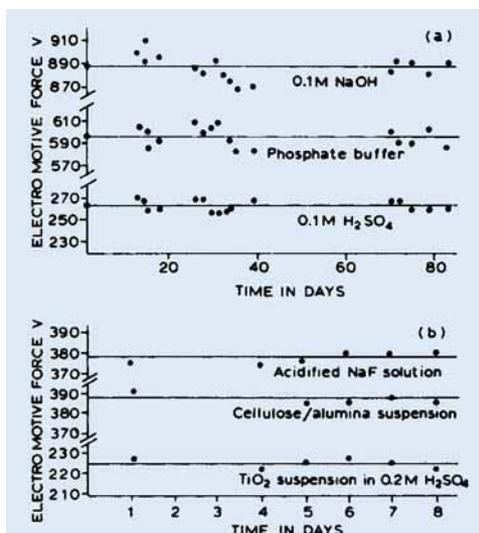
*Fig. 1 (a) The stability of the PallapHode is excellent, with low drift over long periods of time. (b) Even in these aggressive media remarkable stability is achieved over considerable periods of time*
