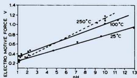
*Fig. 2 With the PallapHode, the linear Nerstian response holds at temperatures as high as 250°C. As far as is known, no other pH sensor can operate over such a wide temperature range*
