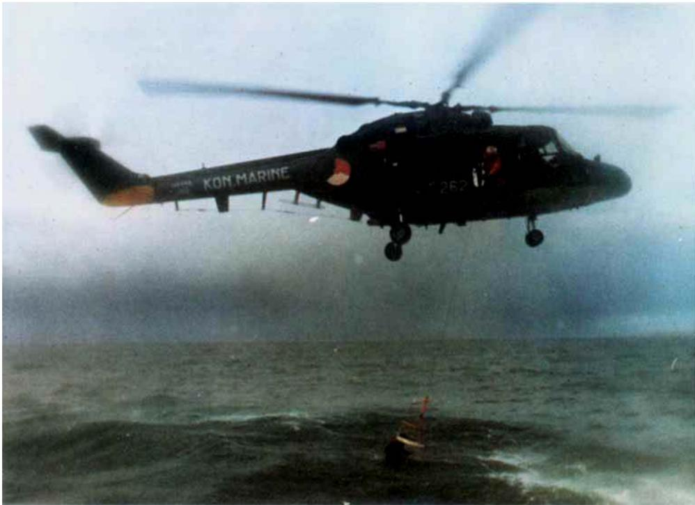
*Fig. 1 A rescue helicopter operating at sea level ingests a high level of salt water into the air intake with resulting contamination of compressor and turbine components by salt residues. During these operations several hours may be spent in such environments*
