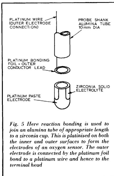
*Fig. 5 Here reaction bonding is used to join an alumina tube of appropriate length to a zirconia cup. This is platinumised on both the inner and outer surfaces to form the electrodes of an oxygen sensor. The outer electrode is connected by the platinum foil bond to a platinum wire and hence to the terminal head*
