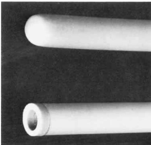
*Fig. 4 Compared with a conventional domed end ceramic sheath (top), the sheath with a platinum foil window (bottom) permits a more rapid response to temperature change*
