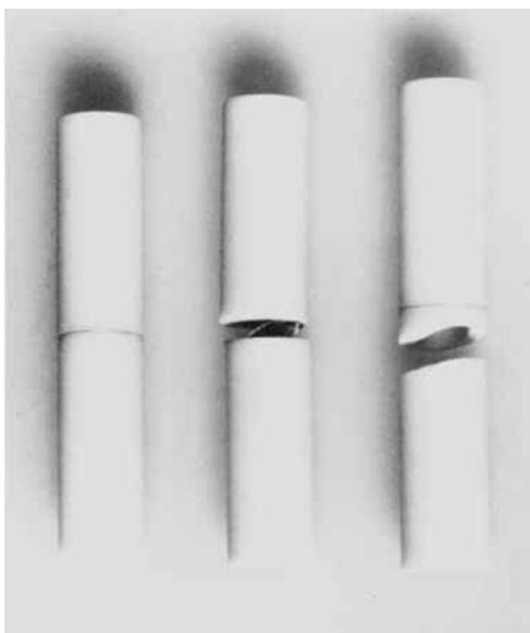
*Fig. 3 Hot modulus-of-rupture test specimens of alumina-platinum-alumina bonds formed in identical conditions. Left: unbroken specimen, middle: specimen fractured through the bond, right: specimen fractured through the alumina*
