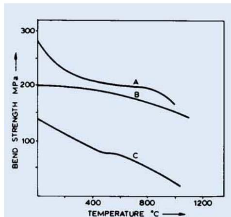
*Fig. 2 Typical mechanical bend strength data for alumina-platinum-alumina bonds over a range of temperatures. Comparable data for commercial alumina, and tensile strength data for platinum are also given.
