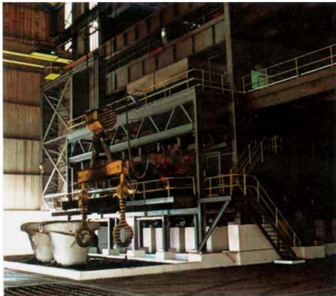
to yield the free mineral particles of platinum generally known as "metallics". The concentrates from which these have been separated, and which still contain some two-thirds of the platinum metals as well as most of the base metals, are further treated by flotation, then filtered, dried, pelletised and smelted to a matte containing mainly nickel and copper sulphides and some 25 to 30 ounces of platinum per tonne.
