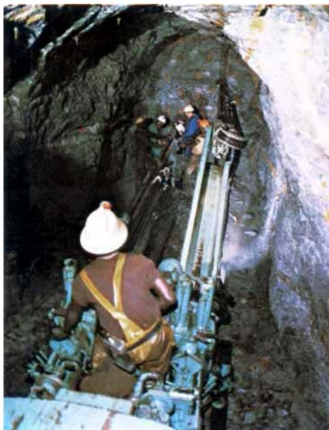
The use of twin-boom pneumatic rigs, for drilling the holes to contain blasting explosives during the development of underground haulage routes allows a considerable saving in labour and improved breaking efficiencies, and has also improved working conditions
