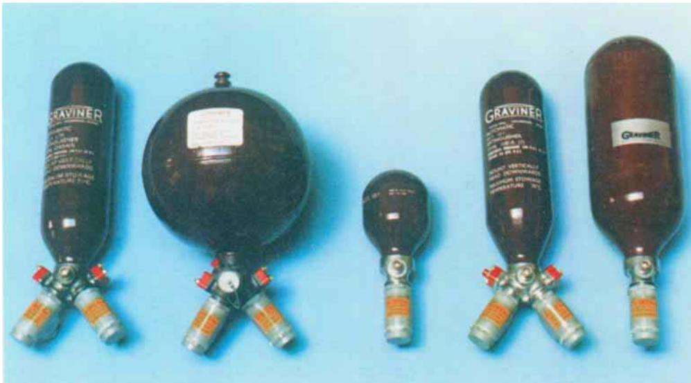
**Fig. 1** Each Graviner aero-engine fire extinguisher is fitted with a bursting disc for either cockpit activation of the unit or protection in case of fire engulfment. Platinum is used as the disc material because of the highly corrosive nature of BCF at elevated temperatures
