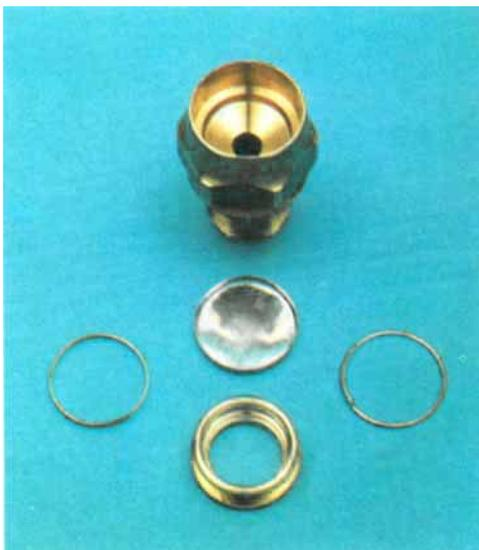
**Fig. 2** The platinum bursting disc is silver brazed into a housing designed to ensure correct location and provide leak-tightness
