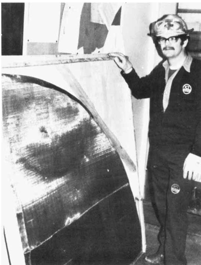
Fig. 5 A folded catchment gauze pack can be delivered in a case not much larger than one quarter of the area of a normal pack, thus facilitating easier storage and transportation, particularly when the latter is undertaken by air
