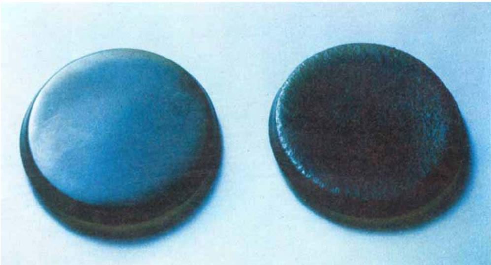
**Fig. 11** XRF sample beads prepared in moulds that have been in service for some time. The bead on the left was prepared in a ZGS 5 per cent gold-platinum mould and shows a good surface finish. The poor surface finish of the bead on the right is the result of excessive grain growth in a standard gold-platinum mould during service; the illustrated surface is also noticeably concave
