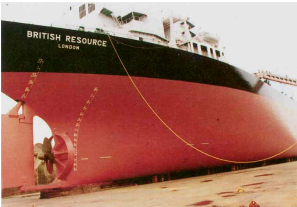
**Fig. 1** Smooth corrosion-free hulls minimise the power necessary to move ships through the water. Modern vessels, such as the tanker illustrated here in dry dock, are in many cases fitted with impressed current cathodic protection methods for corrosion protection. Platinised titanium counter electrodes used in part of such a system can be seen as four small horizontal strips in line with the propeller shaft
