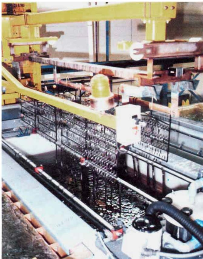
**Fig. 6 Chelated palladium bath with a capacity of 2,250 litres, in automatic plating facility at Speidel Division of Textron, Inc., Lincoln, Rhode Island. This installation is believed to be the largest palladium plating facility in the world**
