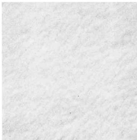
**Fig. 3** This plating was electrodeposited at 200 mA/cm<sup>2</sup> from chelated complex with revised brightener system at a plating temperature of 70°C. With sufficient agitation, crack-free deposits are obtainable at current densities exceeding 500 mA/cm<sup>2</sup>. It should be noted that this photomicrograph is reproduced here at a magnification which is significantly larger than that used for the two previous figures ×7000
