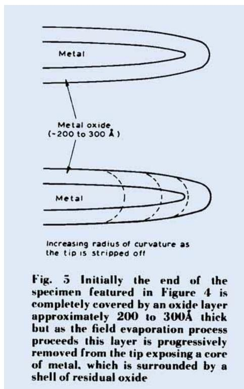
**Fig. 5** Initially the end of the specimen featured in Figure 4 is completely covered by an oxide layer approximately 200 to 300Å thick but as the field evaporation process proceeds this layer is progressively removed from the tip exposing a core of metal, which is surrounded by a shell of residual oxide
