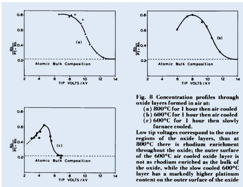
**Fig. 8 Concentration profiles through oxide layers formed in air at:**
