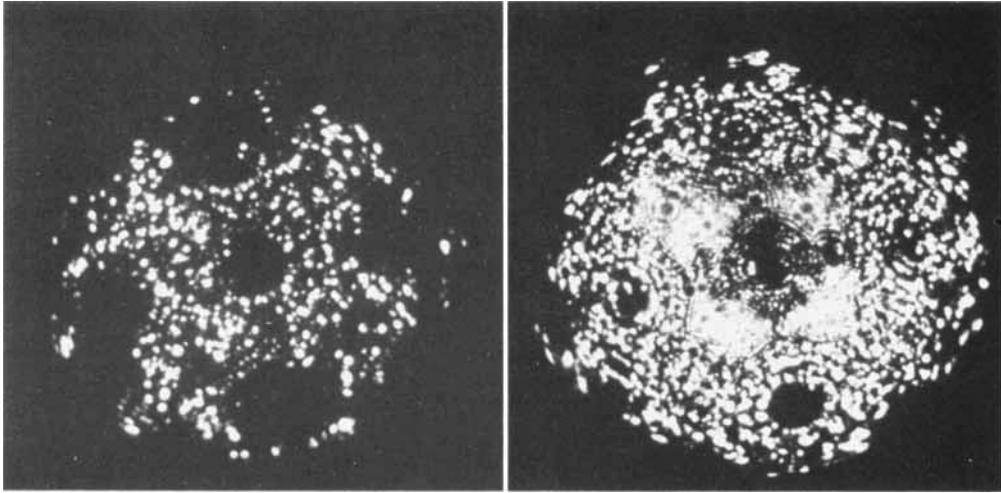
Fig. 6 Treatment at 600°C results in a thinner oxide layer than that produced at 800°C and shown in Figure 4. However, evaporation through the thinner oxide layer shows thermal faceting on (001) and (111) poles. These poles are not imaged initially at 12.0 kV (left), but at 15.75 kV (right) sufficient oxide has been removed to reveal metal around the (001) pole
