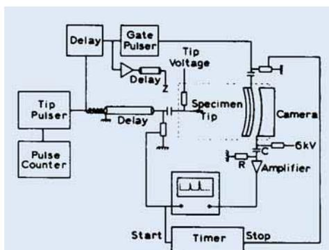
**Fig. 2** In the Imaging Atom Probe the tip of the specimen is arranged at the centre of curvature of a cascade-type double channel plate and screen assembly. The application of a high voltage pulse to the tip of the specimen enables the time-of-flight of the desorbed ions to be monitored, by recording the electrical output signal from the channel plate
