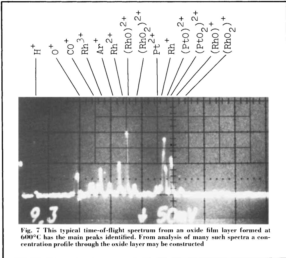
Fig. 7 This typical time-of-flight spectrum from an oxide film layer formed at 600°C has the main peaks identified. From analysis of many such spectra a concentration profile through the oxide layer may be constructed
