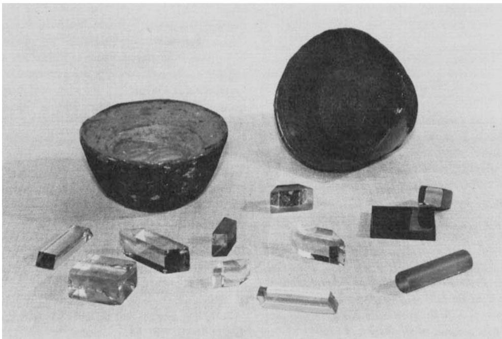
Some of the pieces of optical glass made by Faraday during his investigation of ways of improving the quality of glass for telescopes. The paper presented to the Royal Society described his use of platinum for the construction of vessels and instruments in contact with molten glass and also its use in powder form to eliminate bubbles from the glass
