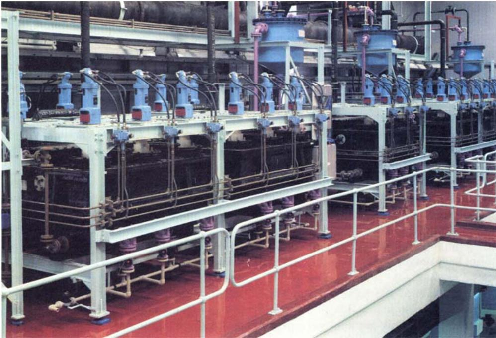
**Fig. 3** After the extraction of gold, iron and tellurium, the platinum group metals are extracted. The separation of platinum, palladium and iridium relies upon a particular metal being selectively extracted from the aqueous phase by an immiscible organic solvent in counter-current mixer-settler boxes
