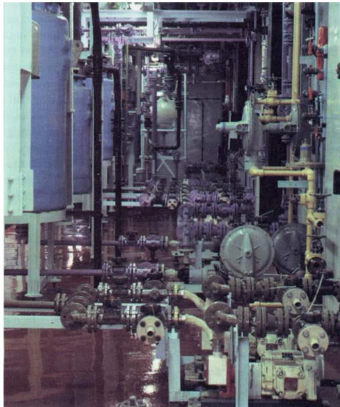
**Fig. 4** One hundred and eighty pumps are used to transfer the liquors through the various stages of the extraction process. The use of closed containers minimises the contact of personnel with process materials
