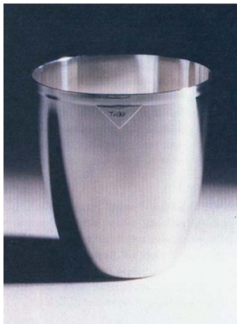
Fig. 2 This laboratory crucible, with a capacity of 30ml, is made from the new Johnson Matthey Metals' composite material ZGS Platinum "TriM". The core of palladium is sandwiched between two layers of zirconia grain stabilised platinum. The latter provides the necessary high temperature strength and resistance to both grain growth and corrosion while the cheaper palladium core gives the good rigidity required for this application
