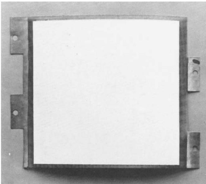
**Fig. 3 Fuel cell electrode showing the nickel mesh current collector and inter-cell connectors. The white porous hydrophobic layer prevents loss of electrolyte from the system while allowing the gases to diffuse to the platinum catalysed layer beneath**
