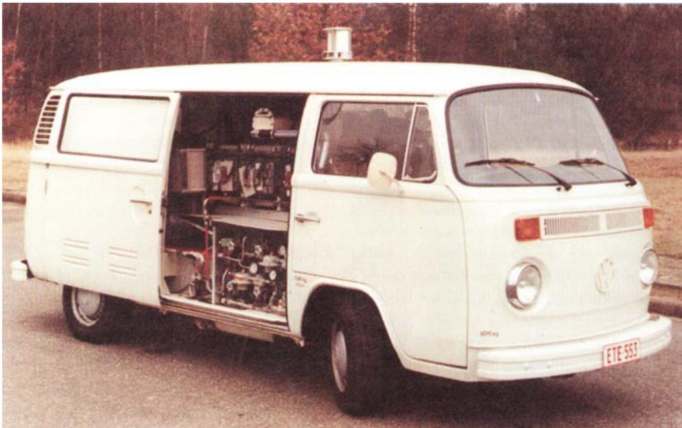
**Fig. 1 This Volkswagen van is propelled by a hybrid fuel-cell battery system and was first used on the road in 1982. Currently it is employed as a mobile test bed. The electrodes of the alkaline fuel cell are catalysed with platinum and the unit is fed with air and hydrogen, the latter being stored in high pressure containers which permit a driving range of 200 km**
