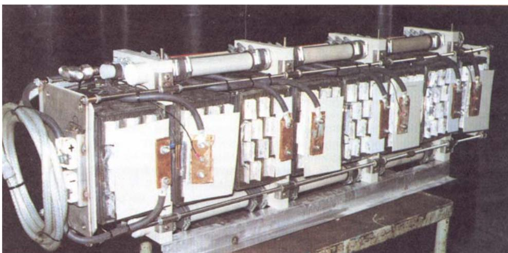
**Fig. 5** Simple connections enable 500 watt fuel cell blocks illustrated in Figure 4 to be built into larger stacks capable of providing proportionally higher power outputs. The assembly shown here has a 4 kW rating, the units sharing common gas and electrolyte supplies
