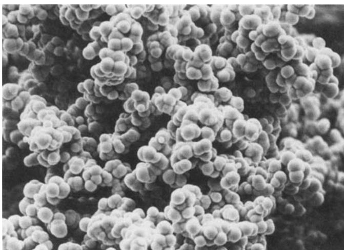
**Fig. 6** Palladium powders used in the manufacture of multilayer ceramic capacitors must be produced to a very high level of purity and to a controlled morphology. This scanning electron micrograph shows a suitable powder consisting of spherical, unagglomerated particles of low surface area and with a particle size between 0.5 and 2 microns
