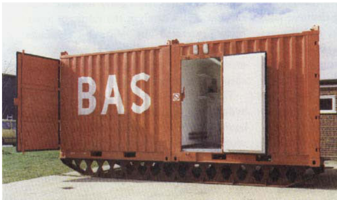
Fig. 3 This containerised methanol/water hydrogen generator has been made for the British Antarctic Survey who will use the hydrogen to fill the balloons that lift sensitive meteorological instruments into the high atmosphere. The caboose is sledge mounted so that the whole self-contained unit can be moved regularly. It is hoped that this will prevent loss of the equipment by burial in heavy snowfalls and subsequent incorporation into the ice cap
