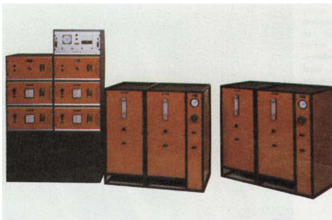
Fig. 2 Two HM2 diffusion units are shown here prior to despatch. In this range the units are supplied as two separate cabinets, one housing the gas purifying system and the other the electrical controls which therefore can be sited well away from the hydrogen gas system. These units provide a simple and economic means of upgrading commercially available hydrogen from a variety of gas sources to the ultra high purity required during the manufacture of semiconductor devices
