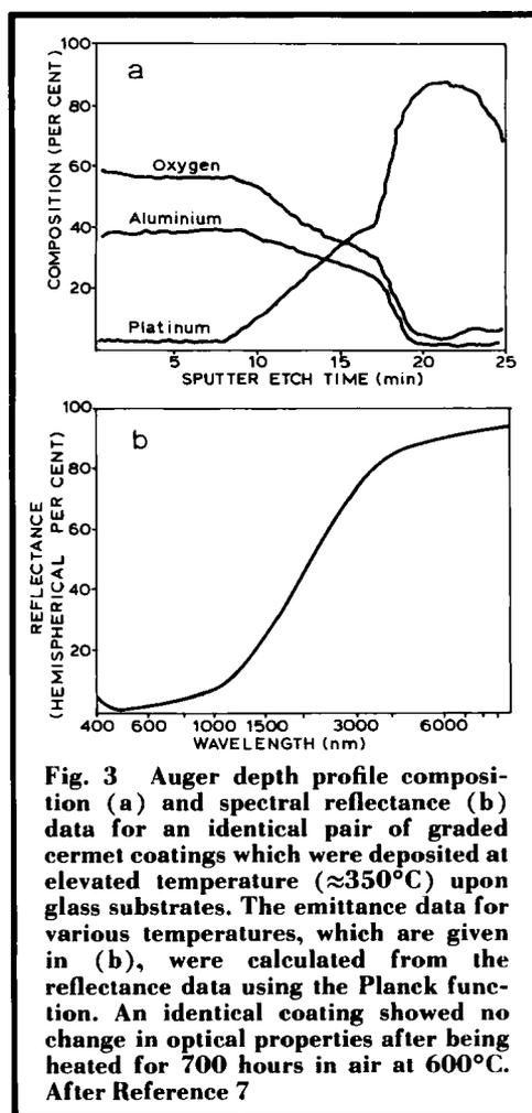
Fig. 3 Auger depth profile composition (a) and spectral reflectance (b) data for an identical pair of graded cermet coatings which were deposited at elevated temperature ( $\approx 350^\circ\text{C}$ ) upon glass substrates. The emittance data for various temperatures, which are given in (b), were calculated from the reflectance data using the Planck function. An identical coating showed no change in optical properties after being heated for 700 hours in air at 600°C. After Reference 7
