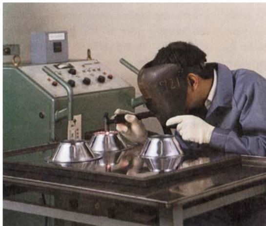
These two illustrations show welding processes during the fabrication of platinum equipment for the glass industry. The chemical and physical properties of platinum and a number of its noble metal alloys make them eminently suitable for this most demanding high temperature application
