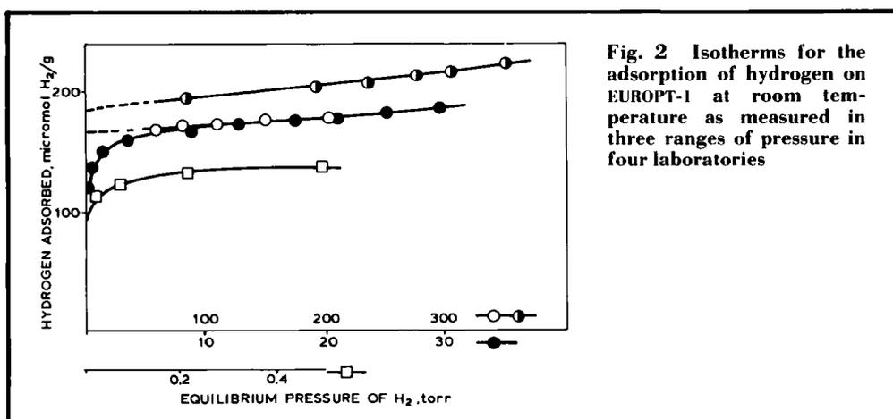
Fig. 2 Isotherms for the adsorption of hydrogen on EUROPT-1 at room temperature as measured in three ranges of pressure in four laboratories
