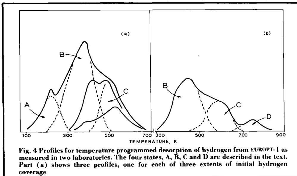
spills back onto the metallic function and undergoes atom recombination to give gaseous dihydrogen molecules. The population of state **B** hydrogen was such that, if the  $H_{\text{adsorbed}}:Pt_{\text{surface}}$  stoichiometry is 1.0:1.0, then the dispersion of the platinum is about 65 per cent, in fair agreement with that obtained by electron microscopy.
