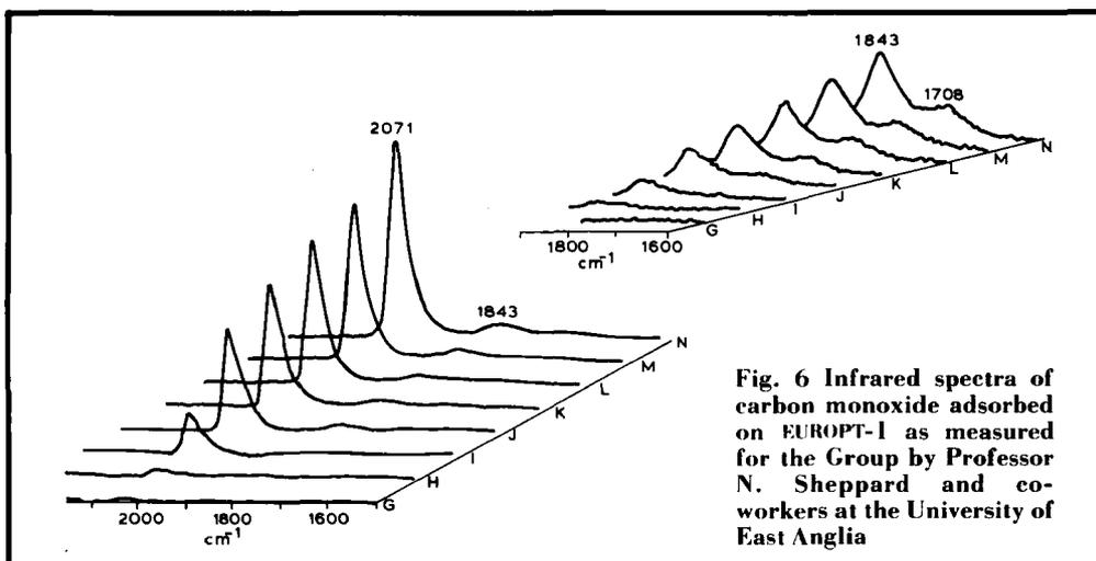
Fig. 6 Infrared spectra of carbon monoxide adsorbed on EUROPT-1 as measured for the Group by Professor N. Sheppard and co-workers at the University of East Anglia
