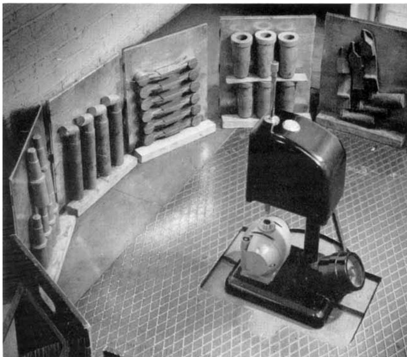
*A portable isotope carrier and time-controlled exposure unit in use for the gamma radiography of a number of copper alloy castings in the foundry of Mallory Metallurgical Products Ltd.*
