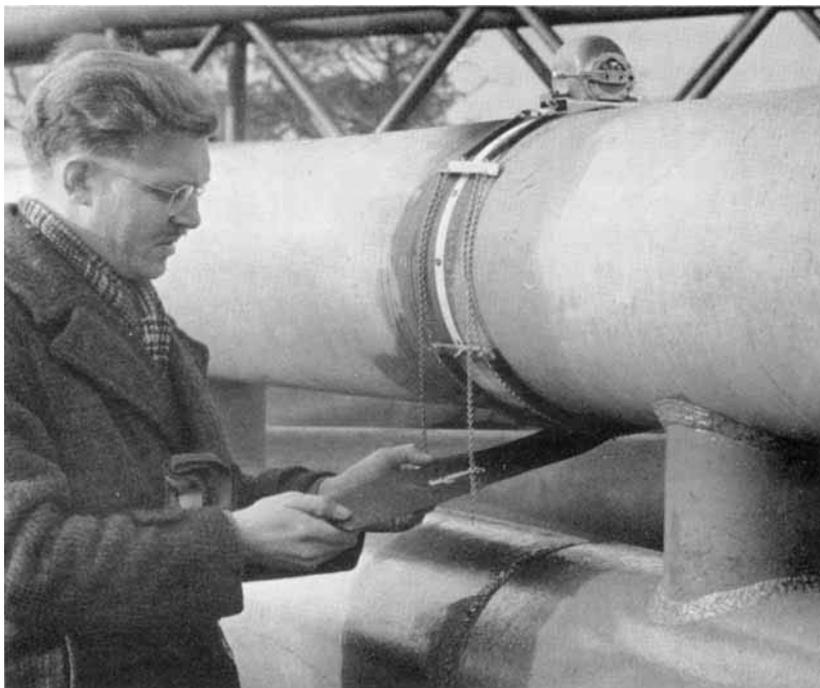
*Gamma ray inspection, using iridium 192, of one of the welds in a tubular steel structure by Stewarts and Lloyds Ltd.*
