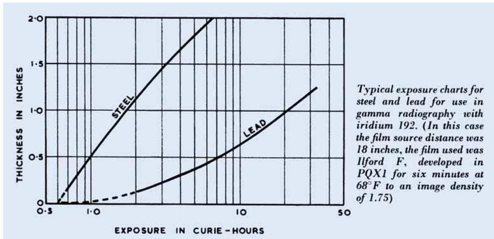
or 400 kV X-rays for detection of fine cracks, but that the flaw sensitivity, when considered in terms of contrast alone, is actually comparable with 400 kV X-rays for thicknesses from 1½ to 3 inches of steel and, although considerably less than that with 200 kV X-rays, remains reasonable for thicknesses down to about ½ inch steel provided that good film processing technique is followed.
