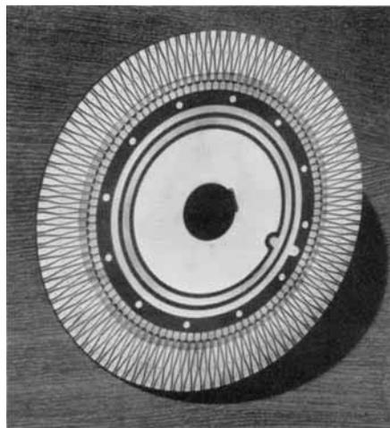
been deposited on the contact surfaces of the 200 sectors as well as on the two slip rings in the centre. Originally the stator had an outside band of copper linking the sectors, as well as a connecting strip to the two slip rings, to permit plating.
