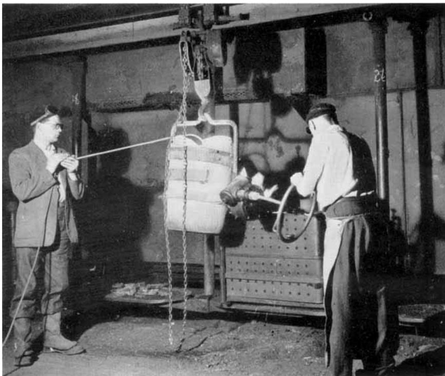
*Measuring the temperature of grey iron while pouring a cylinder block casting in the Dagenham foundry of the Ford Motor Company Ltd. A platinum : 13 per cent rhodium-platinum quick-immersion thermocouple is used*
