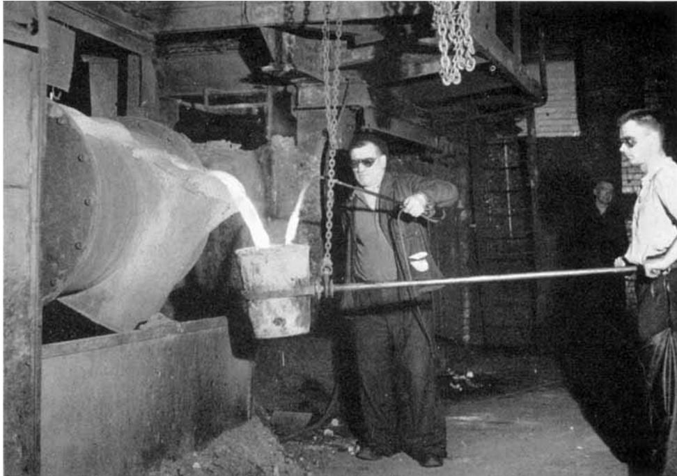
*Taking an immersion reading to determine the liquid alloy steel temperature in the ladle prior to casting crankshafts. The melting process is accurately controlled by taking temperature measurements at five minute intervals*
