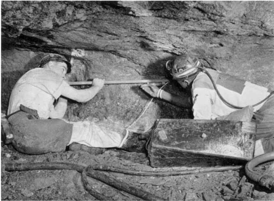
*Charging a hole for blasting on the Merensky reef in the Rustenburg Platinum Mines. The white anorthosite footwall can be seen just level with the miner's knee. Above this lies a thin line of dark grey chromite with an undulating bottom contact. Then follows the coarse-grained pyroxenite of the Merensky reef almost to the roof of the stope, which consists of the less coarse-grained hanging wall pyroxenite*
