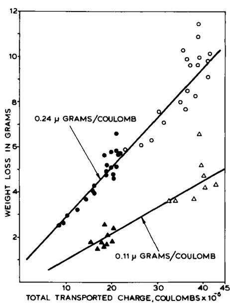
Fig. 14 These plots of mass loss versus electrical charge transported indicate that platinum clad anodes are eroded at a rate of 0.11 μg/coulomb, while those protected by platinum and stainless steel lose metal at a rate of 0.24 μg/coulomb
