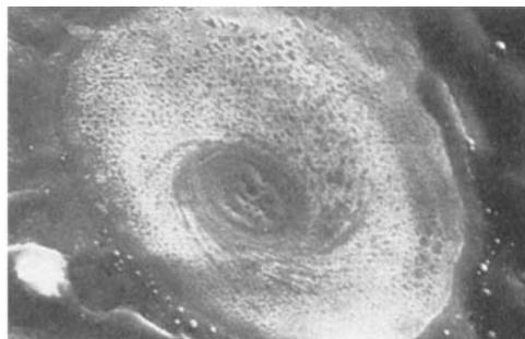
**Fig. 16** An arc termination point on a platinum clad electrode surface again shows melting of the platinum, indicating that this is a cause of platinum loss during power generation. The magnification here is approximately  $\times 1200$ . Reprinted from Reference (5)
