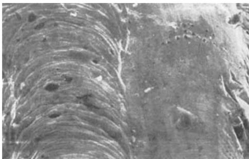
**Fig. 15** This arc track across a platinum clad electrode surface, as seen under the scanning electron microscope, indicates melting of the platinum; the evidence suggests that melting and vaporisation are the major causes of platinum loss. The directions of plasma flow and arc movement are from top to bottom on the micrograph, which is reproduced here at a magnification of  $\times 600$  approximately. Reprinted from Reference (5)
