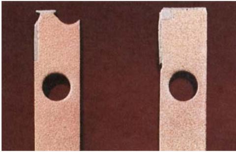
**Fig. 7** In 1978 a significant improvement in anode life was achieved by cladding the upstream edge and anodic surfaces with platinum. These results of a 250 hour test show that the electrode erosion suffered by the earlier design of anode (left) was avoided on the platinum clad modification (right). Plasma flow is left to right
