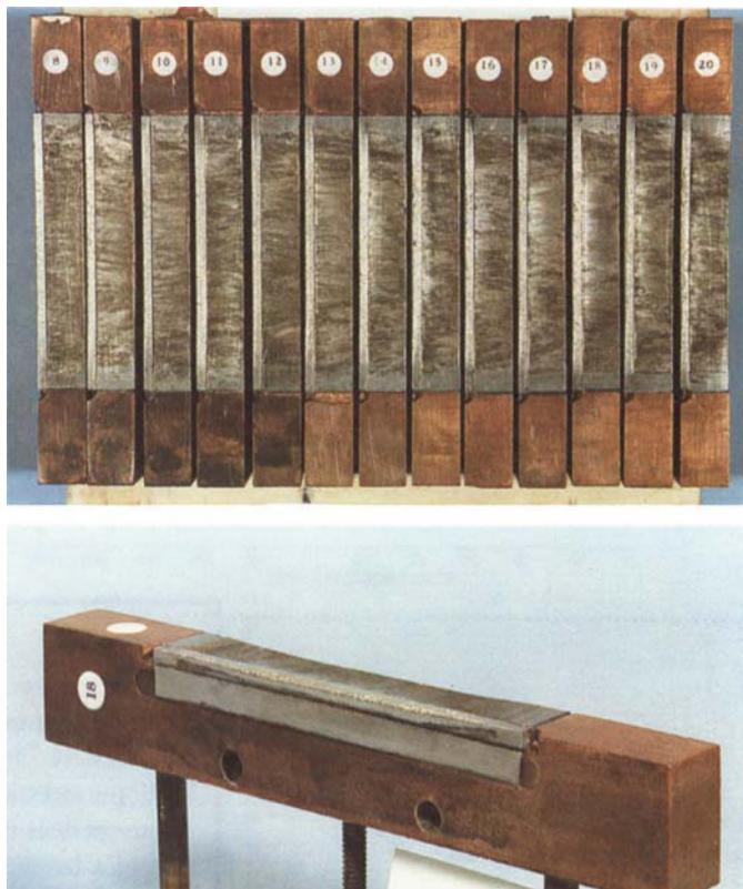
design configurations No. 1 and No. 2 after removal of the slag layer.
