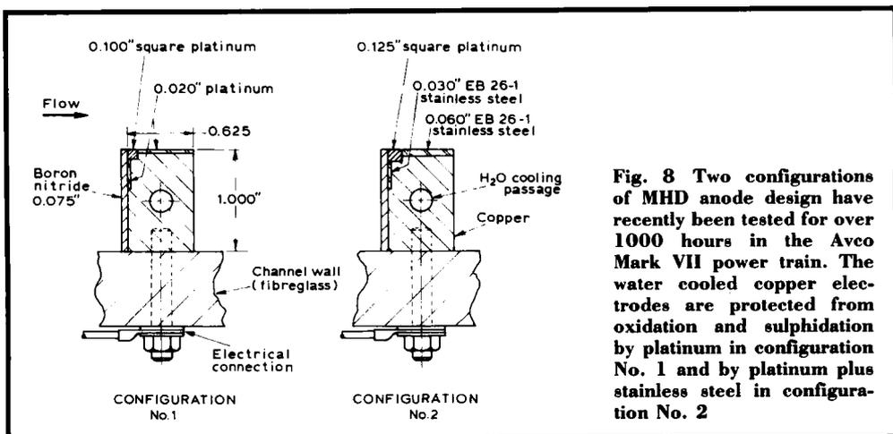
**Fig. 8** Two configurations of MHD anode design have recently been tested for over 1000 hours in the Avco Mark VII power train. The water cooled copper electrodes are protected from oxidation and sulphidation by platinum in configuration No. 1 and by platinum plus stainless steel in configuration No. 2
