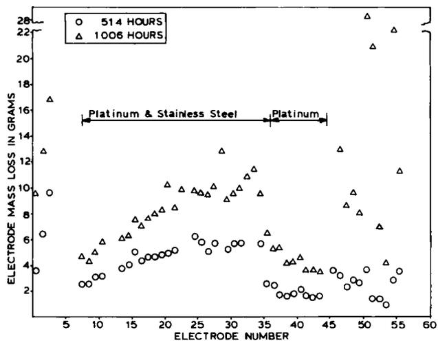
Fig. 13 Except for the two ends of the MHD channel, the mass loss distribution during the 1000 hour test resembles the current density profile, shown previously in Figure 10
