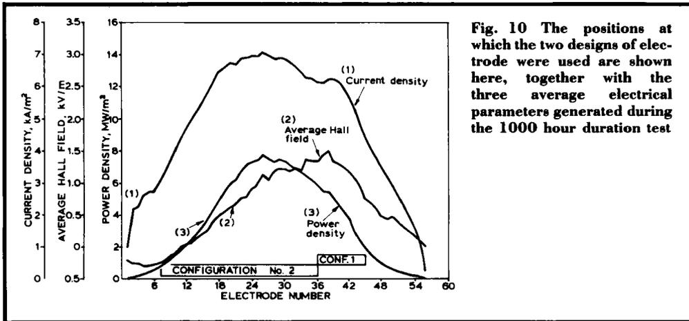
Fig. 10 The positions at which the two designs of electrode were used are shown here, together with the three average electrical parameters generated during the 1000 hour duration test
