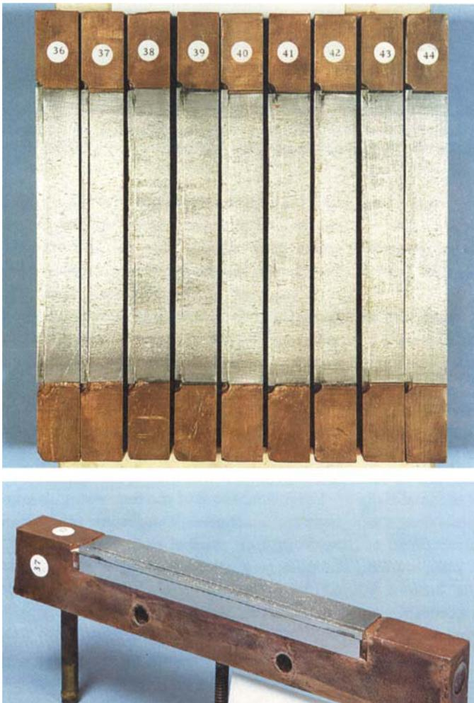
Fig. 11 Magnetohydrodynamic anodes of configuration No. 1 after 100 hours of power generation show that protecting the leading edge and the anodic surfaces with platinum has reduced erosion/corrosion of the anode to levels which suggest that platinum clad anodes could be used under the particularly harsh conditions prevailing in the first (upstream) third of a MHD channel (plasma flowing left to right)
