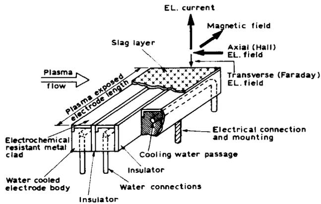
transport of current which can be either diffused or constricted (arcing). Of the two types of electrodes, namely anodes and cathodes (defined as electron emitters), the anodes have proved to be the life-limiting component of the generator and a major design challenge.
