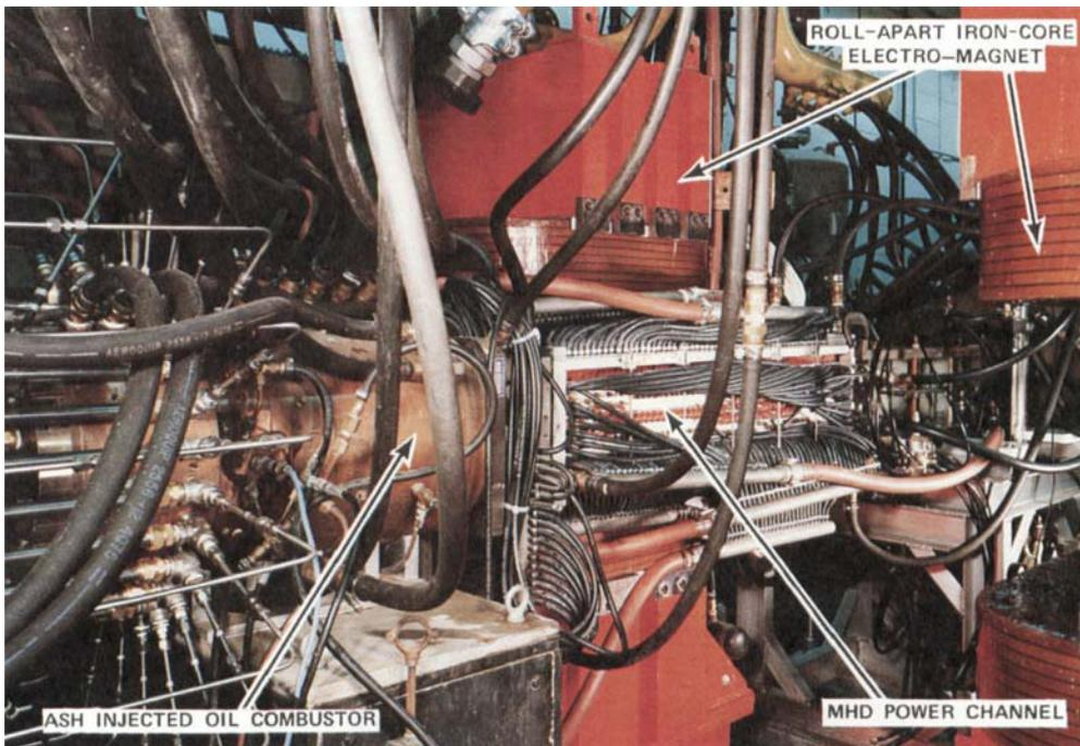
**Fig. 9** The major components of the Avco Mark VII MHD power train are indicated, the 56 pairs of electrodes being located within the one metre long channel which produces a nominal 55kW
