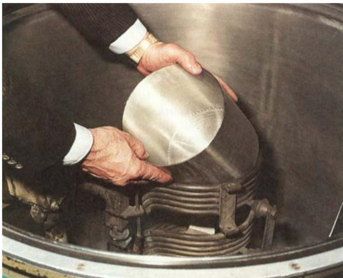
Used for melting the mixed oxides from which gadolinium gallium garnet single crystals are grown, this flat bottomed iridium crucible is one of the larger sizes, having a diameter of 180mm and a capacity of 4330 cc
