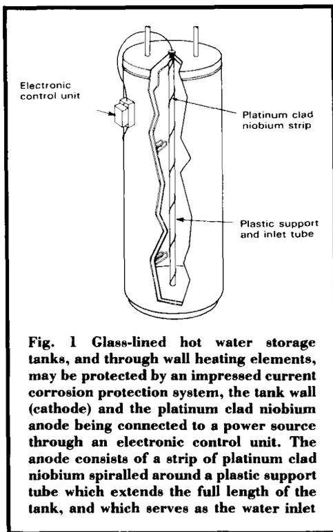
**Fig. 1 Glass-lined hot water storage tanks, and through wall heating elements, may be protected by an impressed current corrosion protection system, the tank wall (cathode) and the platinum clad niobium anode being connected to a power source through an electronic control unit. The anode consists of a strip of platinum clad niobium spiralled around a plastic support tube which extends the full length of the tank, and which serves as the water inlet**
