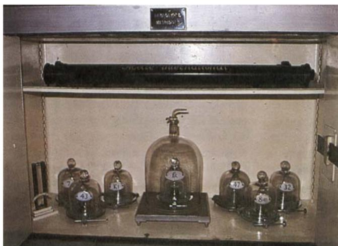
Fig. 1 The International prototype of the kilogram and its six designated copies which are kept at the Bureau International des Poids et Mesures at Sèvres
