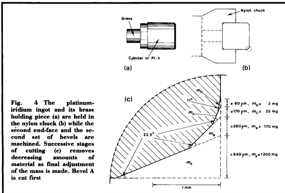
Fig. 4 The platinum-iridium ingot and its brass holding piece (a) are held in the nylon chuck (b) while the second end-face and the second set of bevels are machined. Successive stages of cutting (c) removes decreasing amounts of material as final adjustment of the mass is made. Bevel A is cut first
