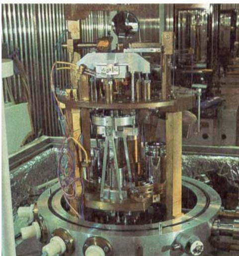
**Fig. 5** The NBS-2 balance at BIPM, with which 1 kg mass standards can be compared to better than 1 part in  $10^9$ . This balance was made at NBS and presented to BIPM in 1970
