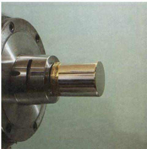
**Fig. 3** This platinum-iridium ingot is still glued to the brass holding piece which supported it in the lathe while final machining of the cylindrical surface and one end-face was carried out
