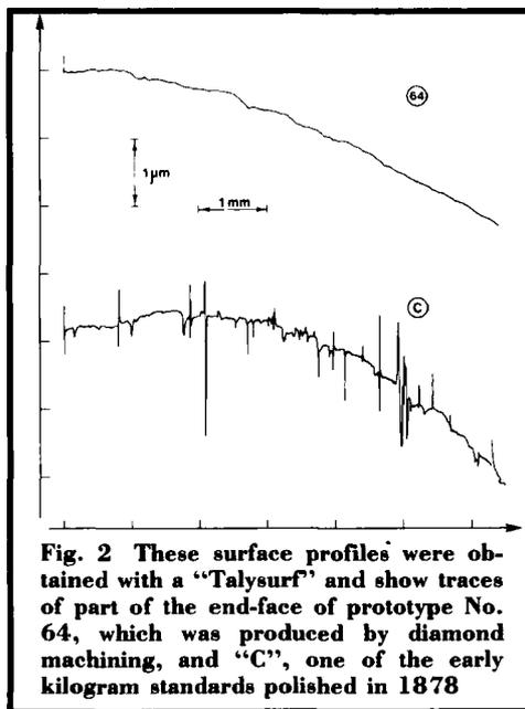
Fig. 2 These surface profiles were obtained with a "Talysurf" and show traces of part of the end-face of prototype No. 64, which was produced by diamond machining, and "C", one of the early kilogram standards polished in 1878
