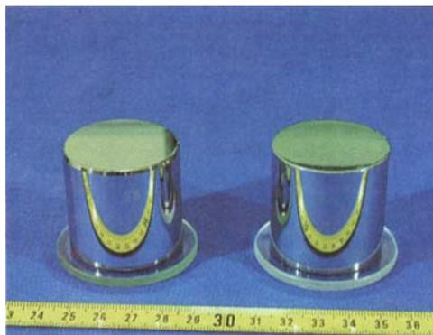
**Fig. 6** A kilogram prototype (No. 68) made using the new diamond machining process (left) and (right) "C" a standard made in 1878
