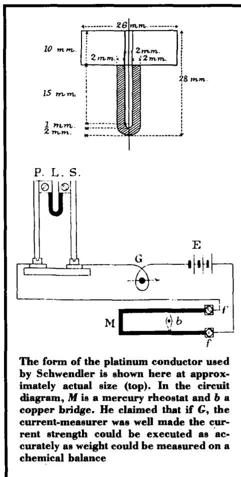
The form of the platinum conductor used by Schwendler is shown here at approximately actual size (top). In the circuit diagram, *M* is a mercury rheostat and *b* a copper bridge. He claimed that if *G*, the current-measurer was well made the current strength could be executed as accurately as weight could be measured on a chemical balance
