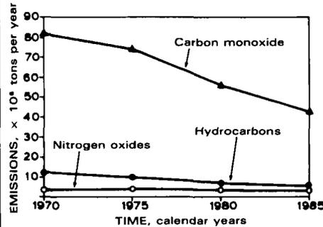
**Fig. 4** The total exhaust emissions between 1970 and 1985 show a considerable fall, even though the total number of vehicles has increased and the total number of miles driven has also increased during this time
