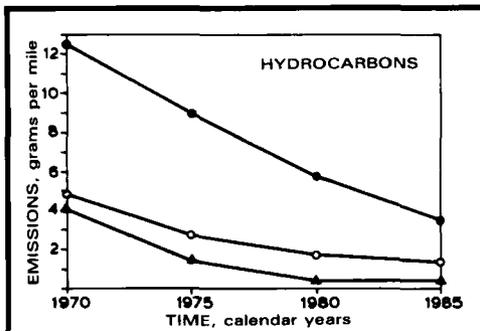
**Fig. 1** The fall in hydrocarbon emissions measured in grams per mile for new cars from 1970 to 1985, after the introduction of the Amendments to the Clean Air Act.
