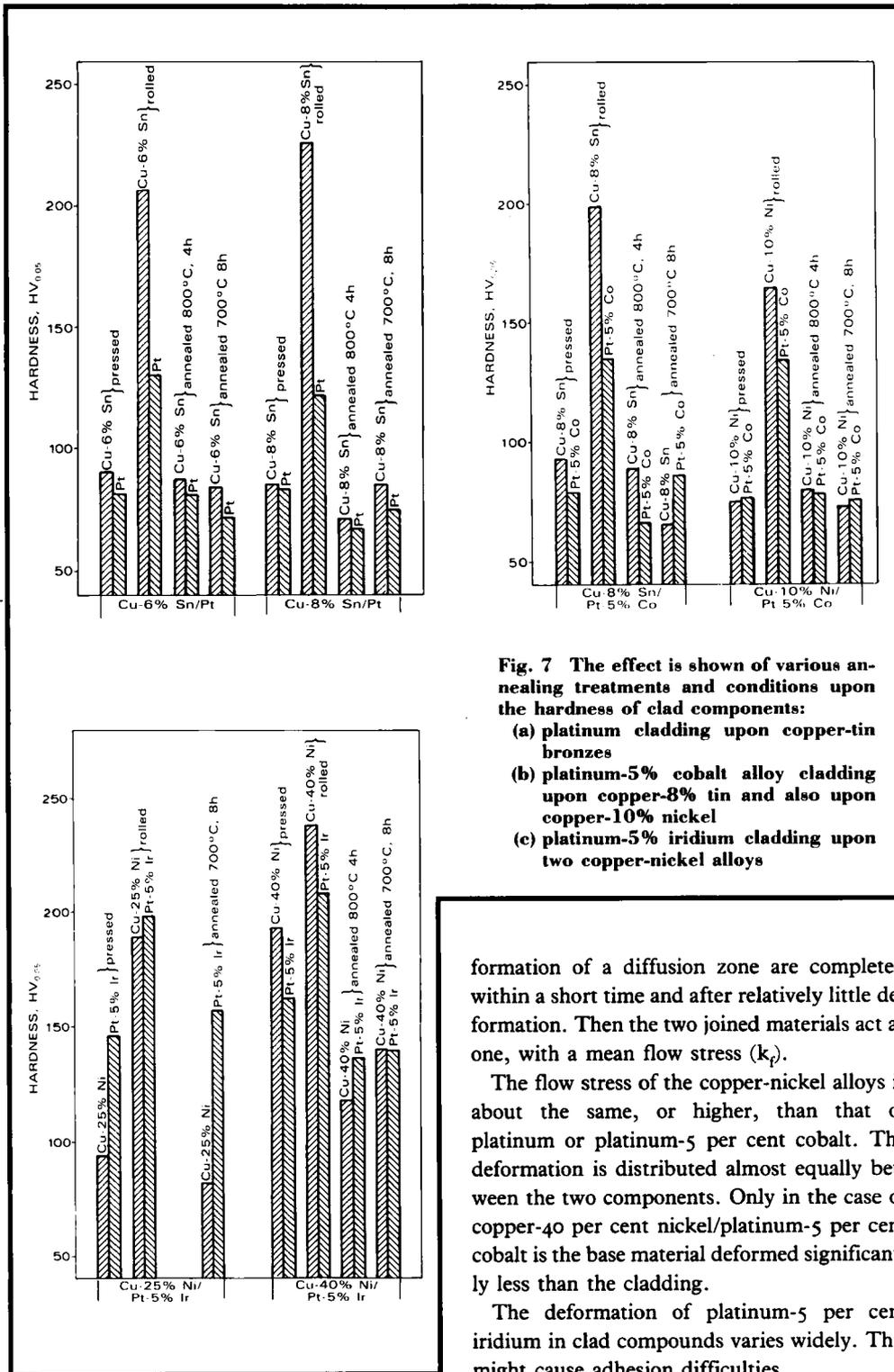
**Fig. 7** The effect is shown of various annealing treatments and conditions upon the hardness of clad components:
