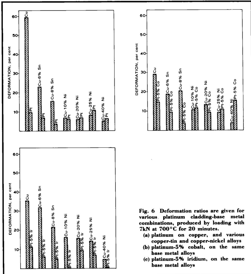
Fig. 6 Deformation ratios are given for various platinum cladding-base metal combinations, produced by loading with 7kN at 700°C for 20 minutes.
