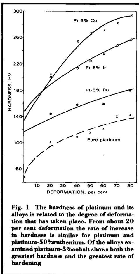
Fig. 1 The hardness of platinum and its alloys is related to the degree of deformation that has taken place. From about 20 per cent deformation the rate of increase in hardness is similar for platinum and platinum-50%ruthenium. Of the alloys examined platinum-5%cobalt shows both the greatest hardness and the greatest rate of hardening
