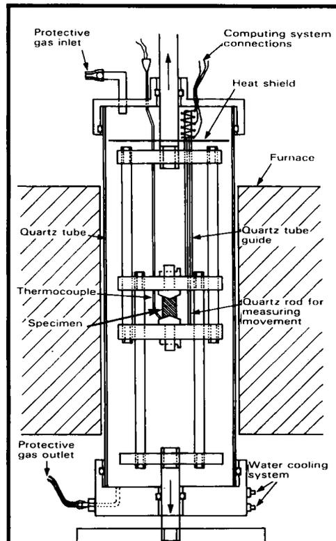
**Fig. 3** Apparatus has been developed to enable the deformation characteristics of the separate and combined materials to be established under various conditions. The main components are indicated here
