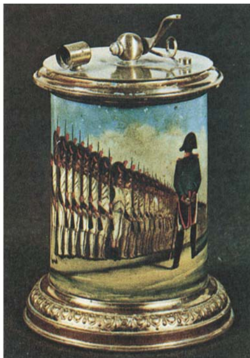
An incidental result of Döbereiner's discoveries was his invention of the first lighter. This employed hydrogen, generated from zinc and sulphuric acid, passing over finely divided platinum which then glowed sufficiently to ignite the gas. A number of different types produced in Germany and in England became very popular and many thousands of them were in use over a long period of time. Many elaborate and fanciful designs on enamel or porcelain were also developed including the two models illustrated here
