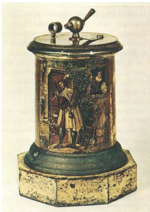
An incidental result of Döbereiner's discoveries was his invention of the first lighter. This employed hydrogen, generated from zinc and sulphuric acid, passing over finely divided platinum which then glowed sufficiently to ignite the gas. A number of different types produced in Germany and in England became very popular and many thousands of them were in use over a long period of time. Many elaborate and fanciful designs on enamel or porcelain were also developed including the two models illustrated here
