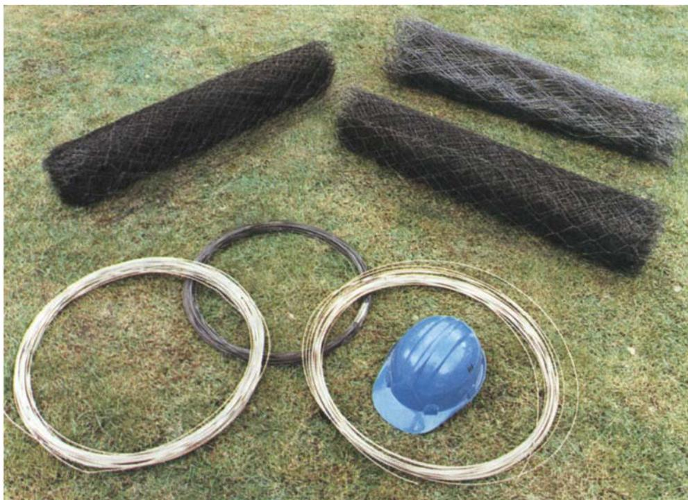
**Fig. 4** These are some examples of the platinised titanium-type materials used in the cathodic protection of reinforcing bars in concrete. The coil of wire at the front right is metallurgically co-processed platinum-clad copper-core niobium (courtesy of IMI Titanium Ltd.). The coil of wire front left is platinum electroplated titanium wire, while the centre coil of wire and the rolls of netting are iridium-based coated titanium (courtesy of Marston Palmer Ltd.)
