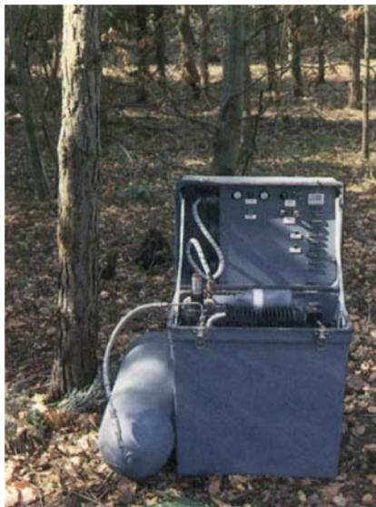
Fuel cell development will be the central feature of the Johnson Matthey display. The 500W prototype shown here has been designed as a portable source of electricity for use in remote locations for charging batteries or for powering communications equipment. The hydrogen fuel is supplied from a lightweight cylinder, but a portable methanol-fuelled generator may be used
