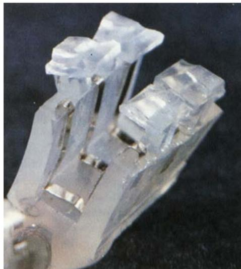
**Fig. 2** This end view of a tripolar electrode group shows the U-shaped platinum electrodes lining a silicon rubber trough where the nerve is placed
