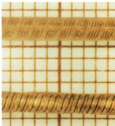
**Fig. 3** The Cooper multiconductor iridium-platinum cable is able to withstand bending, twisting, stretching and crushing, so conforming to the movements of the patient's body. The lower of these two pieces of four-cored cable is an experimental length with colour coded conductors. The sides of the background squares measure 1 mm
