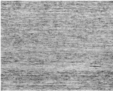
**Fig. 4** The fibrous structure of ZGS 5 per cent rhodium-platinum is retained after annealing at 1100°C, following cold working to a 90 per cent reduction in cross-sectional area × 150
