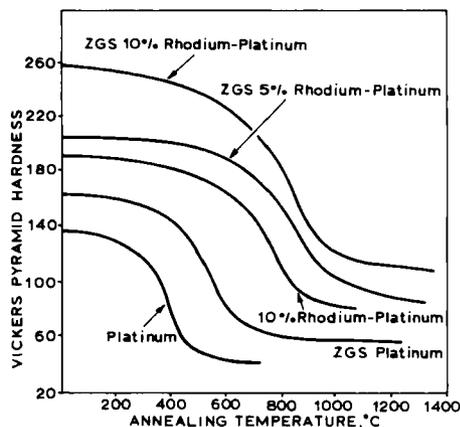
**Fig. 3** Recrystallisation curves are shown for both conventional and zirconia grain stabilised platinum, and some of its alloys. The test samples were held at the annealing temperatures for 30 minutes
