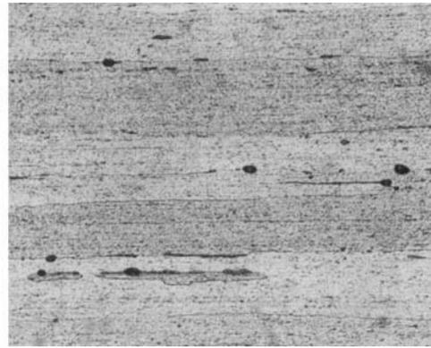
**Fig 5.** Metallographic examination shows that even after prolonged heat treatment at 1400°C ZGS 5 per cent rhodium-platinum retains a fibrous grain structure × 150
