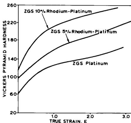
**Fig. 2** Plotting true strain against hardness shows that the work hardening characteristics of ZGS 5 per cent rhodium-platinum are also between those of ZGS platinum and ZGS 10 per cent rhodium-platinum
