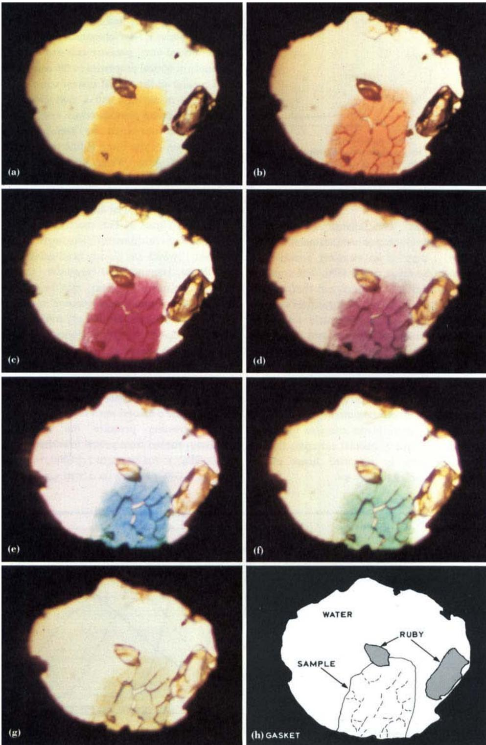
**Fig. 4** The series of photographs on the facing page shows the colour of a thin film of Pd(niox)<sub>2</sub> at various pressures between 0.2 and 10 GPa: (a) 0.2 GPa, (b) 1 GPa, (c) 2 GPa, (d) 3 GPa, (e) 4 GPa, (f) 6 GPa and (g) 10 GPa; the line drawing identifying the position of the palladium complex and the two reference rubies. The aperture in the gasket measures 0.3 mm from side to side
