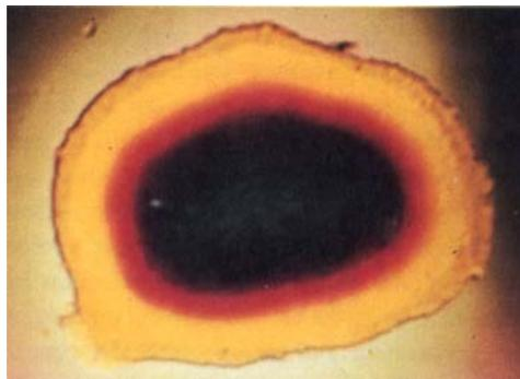
Fig. 5 A pressure gradient produced under non-hydrostatic conditions is displayed visually by the change in the colour of the sample: centre (green) about 6 GPa, middle (red) about 2 GPa, outside (yellow) 0–1 GPa
