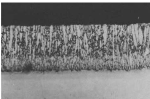
**Fig. 4** This interface between platinum and electrodeposited nickel shows no hole formation after annealing for 8 hours at 700°C  $\times 125$
