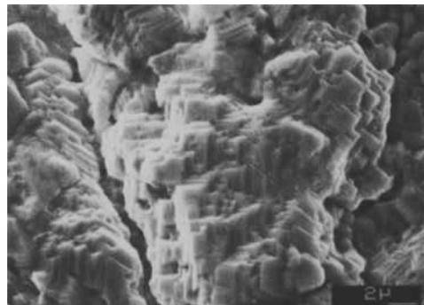
**Fig. 2** The surface shown is that of platinum which has parted from the copper, to which it had been roll bonded, following annealing at 900°C for 48 hours
