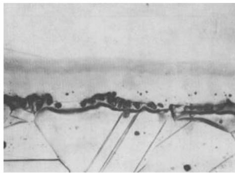
**Fig. 6** After 50 per cent cold deformation followed by annealing for 4 hours at 800°C a porous zone, resulting from the Kirkendall effect, is shown in a platinum-5 per cent cobalt/copper-8 per cent tin diffusion couple  $\times 275$
