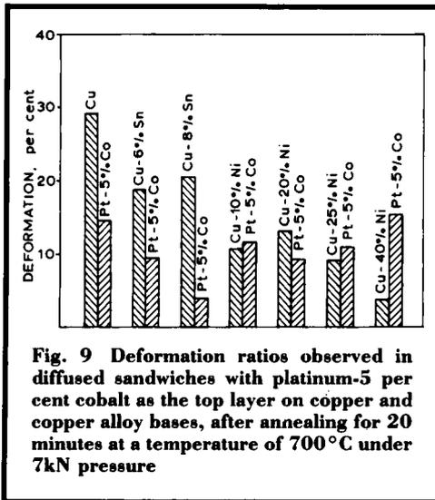
of platinum-5 per cent cobalt to copper or copper-tin alloys by welding are due to excessive void formation in the diffusion layer, resulting from the Kirkendall effect.
