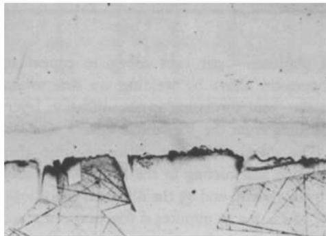
**Fig. 7** After 50 per cent cold rolling followed by annealing at 700°C for 8 hours the porous zone in this platinum/copper-8 per cent tin diffusion couple is thinner than that shown above in Figure 6  $\times 275$
