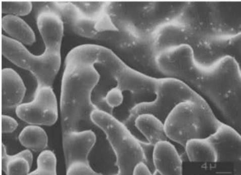
**Fig. 1** When a sandwich of platinum-5 per cent iridium/copper, formed by cold rolling, was annealed for 72 hours at 800°C separation occurred. Scanning electron microscopy showed that the two surfaces which were originally in contact had now developed characteristic forms. The copper side of the diffusion zone is shown above in both electron micrographs, the magnification of both being indicated
