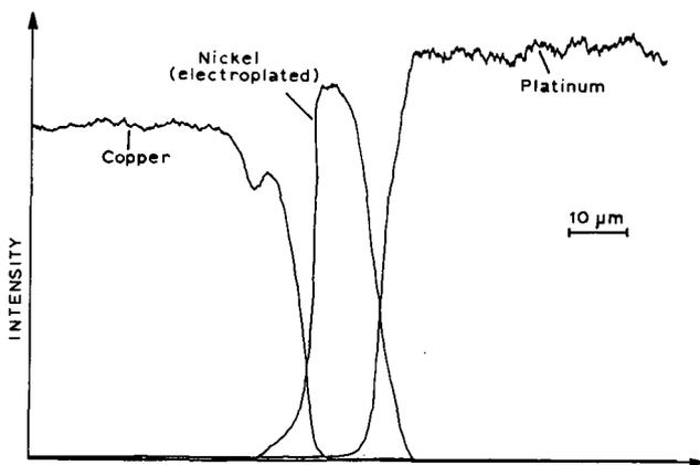
Fig. 14 The concentration/distance profiles of a diffusion zone for a pressure welded copper/electroplated nickel/platinum sandwich are shown after 50 per cent cold rolling and annealing at 700°C for 8 hours. The dip in the copper curve is due to the porous zone
