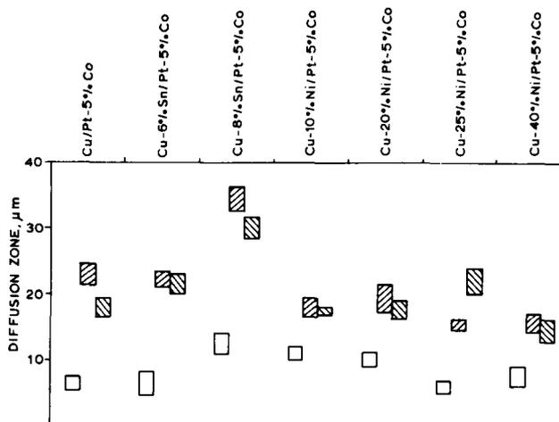
**Fig. 11** Diffusion zone thicknesses are shown for sandwiches of platinum-5 per cent iridium on copper and copper-based alloys after cold rolling and annealing
