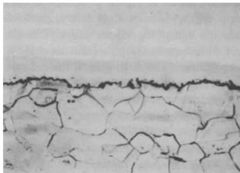
**Fig. 8** Following 50 per cent cold deformation and annealing for 8 hours at 700°C the diffusion zone of this copper-20 per cent nickel base and platinum-5 per cent cobalt top layer contains a zone of porosity, but this is narrower than those shown in Figure 6 and 7  $\times 275$
