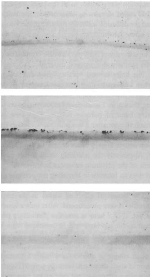
**Fig. 5** Unetched microsections showing the diffusion zones produced when sandwiches of noble metal and base have been annealed at 700°C for 20 minutes under 5kN pressure, followed by cooling to normal pressure. The platinum-rich layers are on top in each case  $\times 275$
