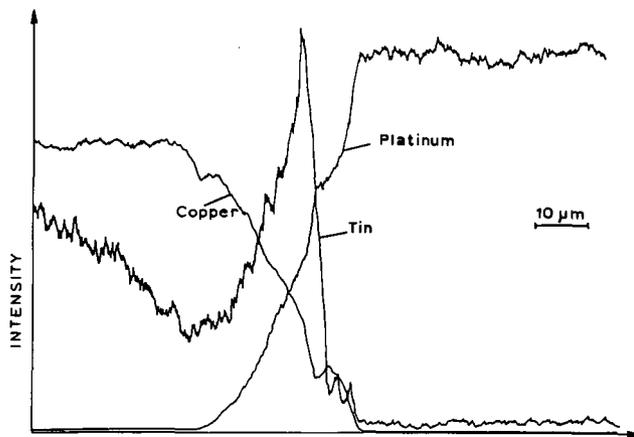
Fig. 12 Shown here are the three concentration/distance profiles across a diffusion zone of a pressure welded 50 per cent cold rolled platinum/copper-8 per cent tin sandwich after annealing at 800°C for 4 hours
