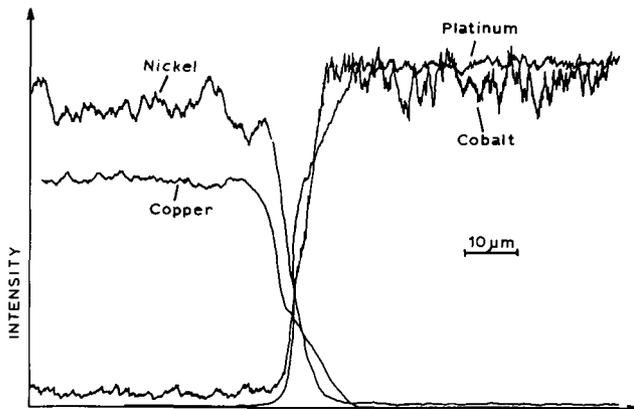
Fig. 13 These are the concentration profiles across the diffusion zone of a pressure welded platinum-5 per cent cobalt/copper-25 per cent nickel sandwich 50 per cent cold rolled after annealing at 700°C for 4 hours. The concentration gradient for copper is much flatter than that of platinum
