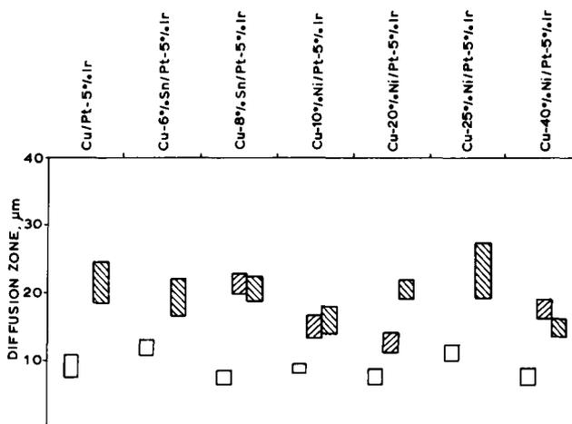
higher nickel concentrations. In general there is less diffusion after 8 hours at 700°C than after 4 hours at 800°C.
