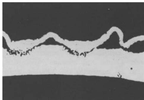
**Fig. 3** Different diffusion rates have caused partial separation of the platinum layer from the copper base. The volume of the platinum has been increased and there is a zone of voids within the copper ×55
