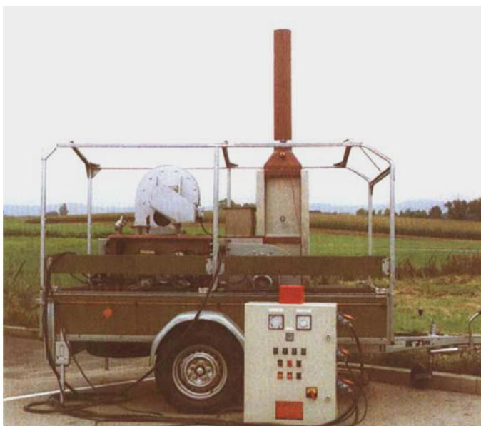
**The Honeycat® mobile pilot unit is designed for a full site trial, and once located close to the process gas outlet it only requires connection to an electricity power supply**
