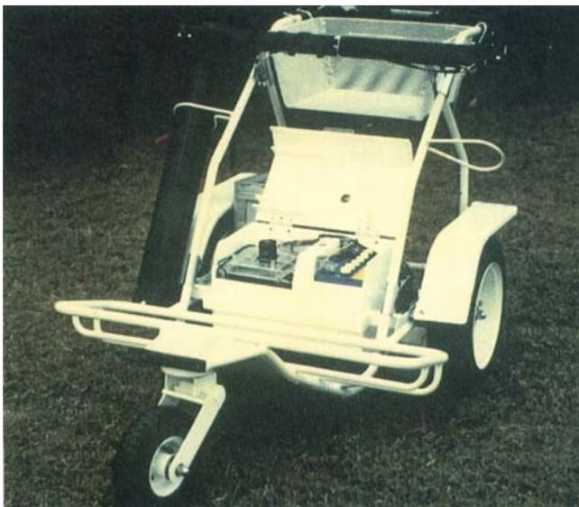
**Fig. 1** Many of the potential applications of direct methanol fuel cells are in domestic and leisure markets. Hitachi have constructed a golf cart with a direct methanol fuel cell in a hybrid system alongside a lead acid battery
